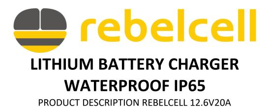
The 12.6V20A Lithium battery charger waterproof (IP65) has been specially engineered to charge the 12V50 AV and up Rebelcell li-ion batteries. The specially designed charging programme ensures that your battery is charged safely and automatically with the correct charging profile (voltage / charging current). The charger shuts off automatically when the charging process is completed.
